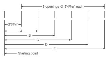
Give the dimensions from column center to the center of each of the anchor bolts marked A, B, and C in this 12" channel.
