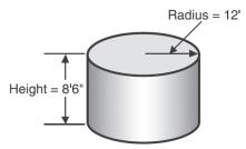
The tank in the previous problem is 90% full of water. How many gallons of water would need to be added to fill the tank?
