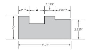
The following figure is an end view of a turned metal shaft. What is the diameter of the smallest circle?
